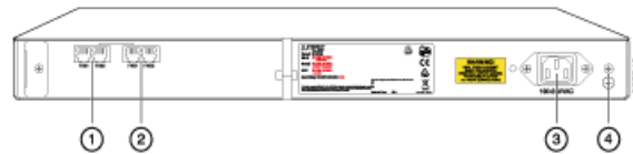
Figure 5: J-SRX240 Services Gateway with Integrated Convergence Services Back Panel
